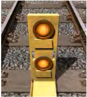
Exit from the worksite
