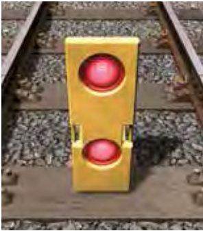
Entrance to the worksite
